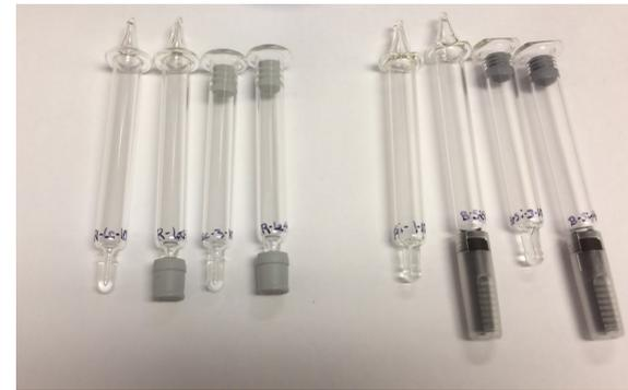
Figure 2. Sample syringes showing how various parts of the syringe can be isolated for study of oxygen ingress. Two types of syringes were studied (staked needle and Luer tip) as well as negative controls (completely flame sealed) and positive controls (flame sealed with micron size laser drilled defects)
